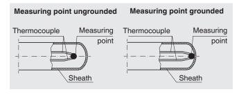
The thermocouple will be delivered as a single thermocouple with an ungrounded measuring point, unless explicitly specified otherwise.
